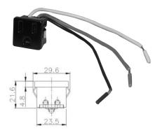
(mounting hole: 1.18" x 0.94") 6" - 16 awg. wire leads terminal **No. 8545**
